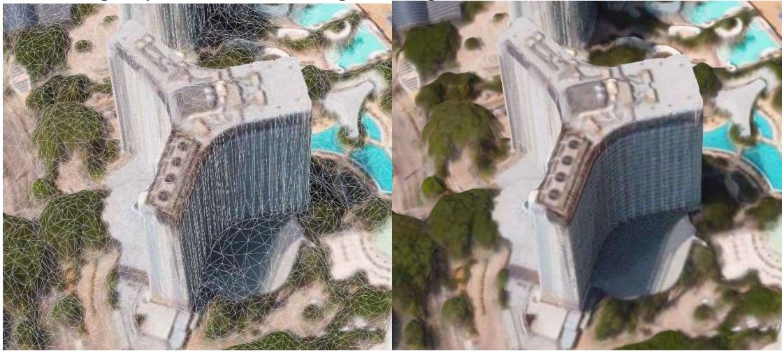
Fig 2: Current 50 cm 3D model; left with overlaid mesh structure
