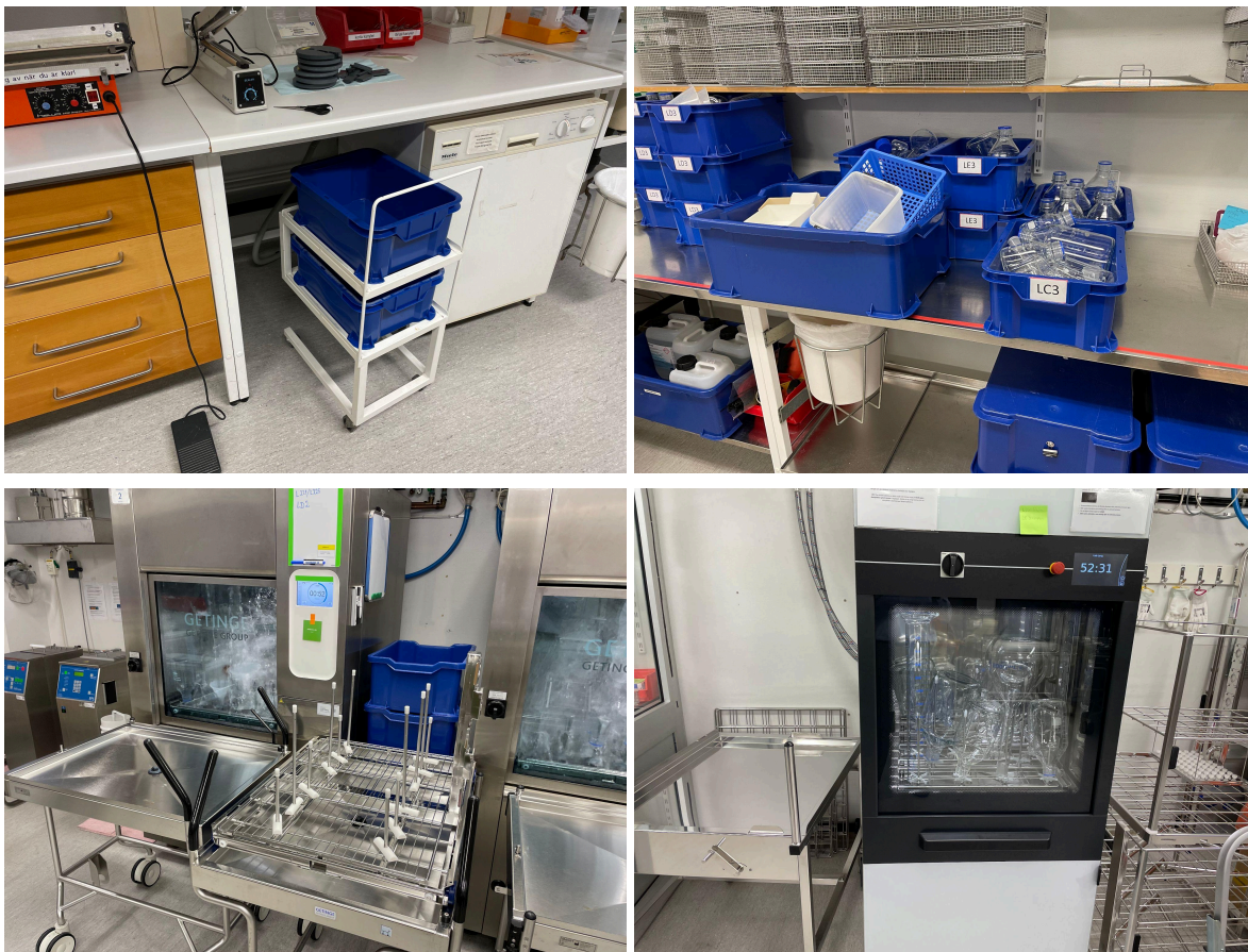
Figure: A cart (top left) is used to transport glassware that needs washing (top right) to a dishwashing area. The glassware is to be loaded onto a dishwashing rack (bottom left) and into an industrial dishwasher (bottom right).
