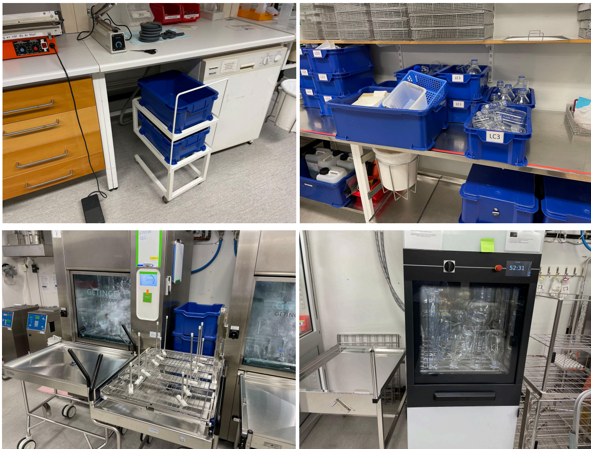
Figure: A cart (top left) is used to transport glassware that needs washing (top right) to a dishwashing area. The glassware is to be loaded onto a dishwashing rack (bottom left) and into an industrial dishwasher (bottom right).
