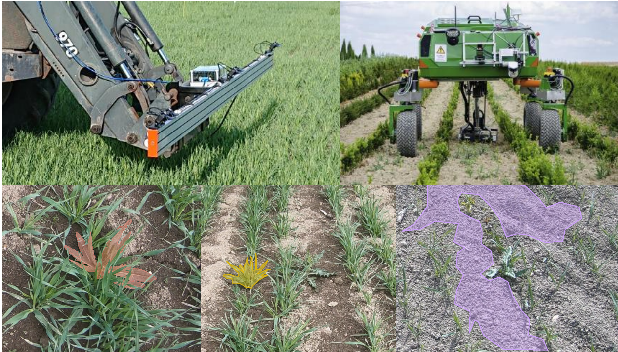
Top row: Cameras mounted on a tractor, and example weeding robot. Bottom row: example details from annotated frames.
