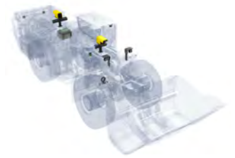
An autonomous Epiroc loader equipped with two lidars, an odometer and an IMU. (Asset: Epiroc)
