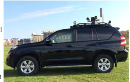
Figure 1: Sensor platform for data collection and real-time execution of positioning algorithms.
